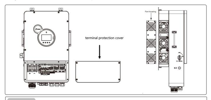
When using the device in areas with poor air quality, the dust screen is easily blocked by air particles. Please disassemble and clean the dust screen periodically to avoid affecting the internal air flow rate of the inverter, which may trigger an over-temperature protection fault (19/20 fault) affecting the use of the power supply and the service life of the inverter.
